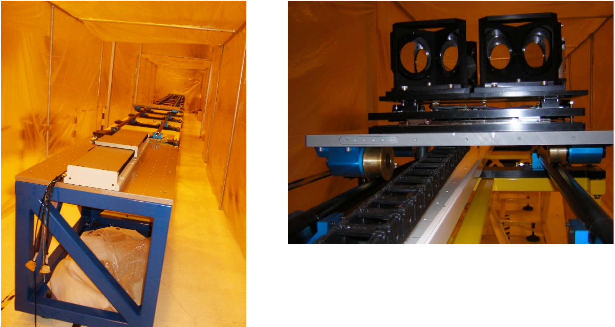
Figure 6: Views of the delay line during the integration phase in Meudon. Left: mechanical structure in the integration tunnel before integration of optics. The translation stage on the front optical table is the Aerotech 1 m stroke stage. The total length of the delay line is 14 m. Right : view of the central carriage with the four dihedrals.
